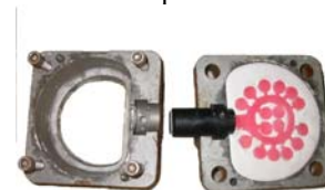
Production of acrylic resin discs in a dental flask.
